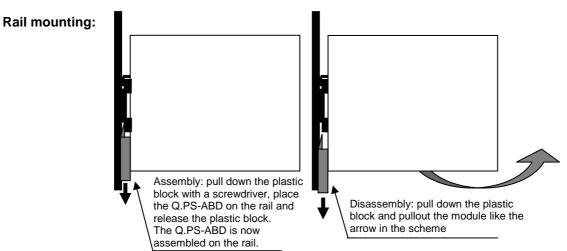
Other modules must have a minimum vertical distance of 10 cm to this power supply in order to guarantee sufficient auto convection.
