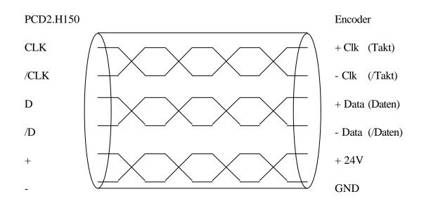
To prevent perturbation problems a shielded and pair twisted cable should be used and the shield should be connected to ground on both sides.
