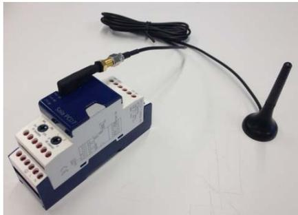
RF-modem with the adapter and the external antenna PCD7.K840
