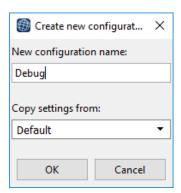
Once the different configurations defined, you can select the configuration from the toolbar. In this way you can easily switch between the different configurations without having to adjust other parameters or settings.
