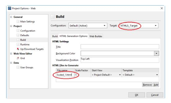
It is necessary to specify the name of the HTML file to generate, the scale factor, the start view and the template. You can add an entry using the 'Add' button at the bottom of the dialog box. At least one entry has to be defined in order to avoid compilation error.
