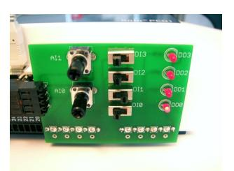
Switch DI0 can now be used to switch digital output DO0
