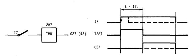
In case of the switch-on delay the timer is also started by the rising edge of I7 as in case of the fleeting-on delay. However, output 27 should be switched on only after the time has elapsed.
