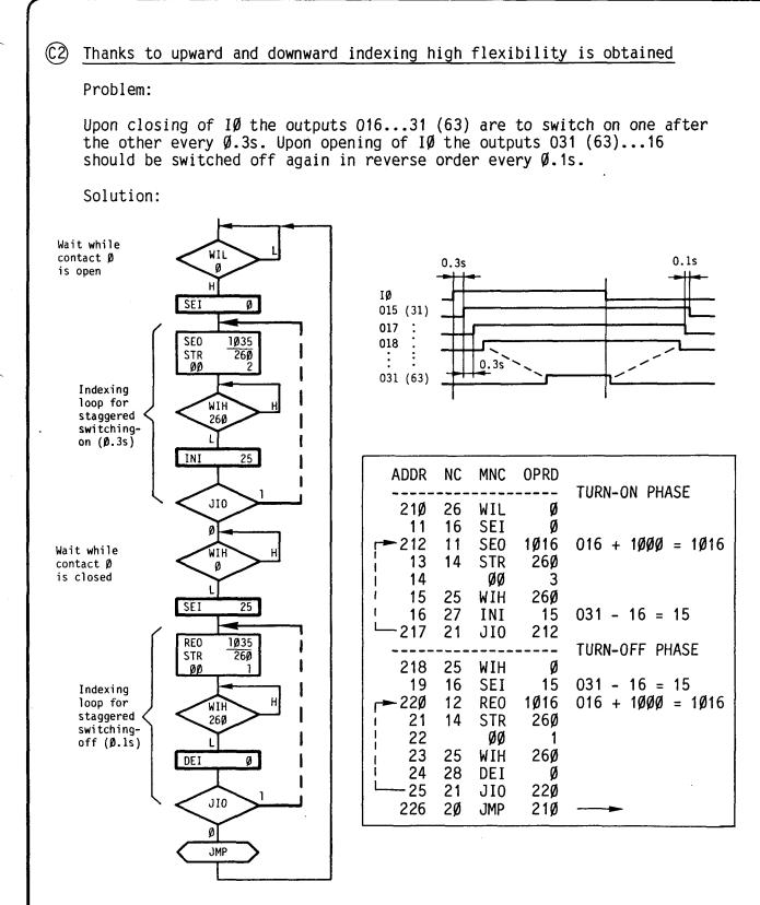
The upper indexing loop is very similar to that in example C1. In the lower loop the index register is set to 15 first. In the first run REO  $1\emptyset16 - 1\emptyset\emptyset\emptyset + 15 = \text{REO }31$  acts upon output 31. The instruction **DEI (28)** decrements the value of the IR by 1, as a result of which output  $3\emptyset$  is switched off in the next run, etc. As soon as the IR =  $\emptyset$ , no further return is effected, the indexing loop is left.
