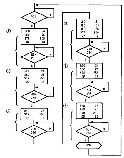
The flow-chart shows the program sequence without subroutines. The program parts which are marked with the brackets are repeated 6 times. Therefore, it is of advantage to write them as subroutines.
