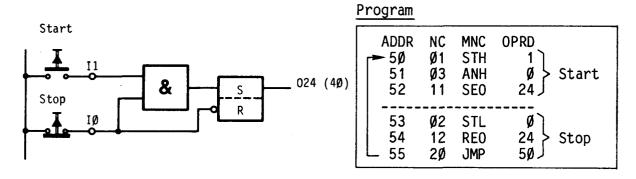
SEO (11): Set Output With this instruction an element (output or flag) is continuously set until it is reset with REO.
