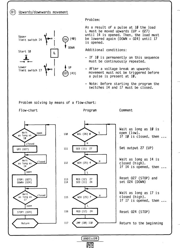
As evident from the example, a sequence is described step-by-step when programming according to a flow-chart. The stages of the process are split up into conditions (wait for an input state) and actions (set or reset outputs).
