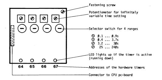
This module is an option and must be ordered separately. It allows easy setting of four time ranges in the RUN-mode independently of the program (e.g. for setting delay times).
