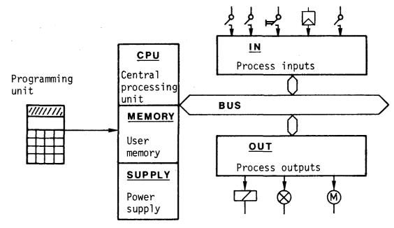
The programming unit serves to transfer the user program to the user memory (RAM). The CPU executes this program, interrogates the states of the process inputs and controls the process outputs accordingly.
