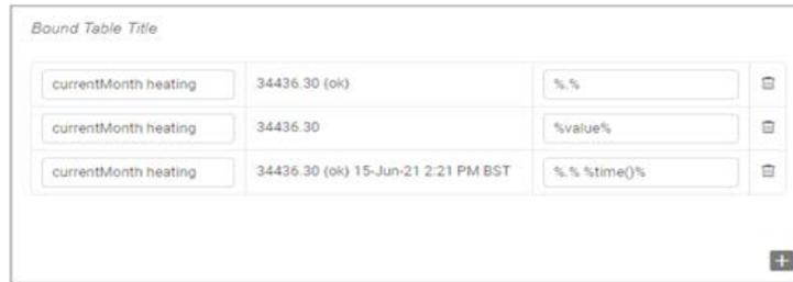
A screenshot of a 'Bound Table' widget in design mode. The table has three rows and three columns. Each row has a 'currentMonth heating' label in the first column, a numerical value in the second column, and a format string in the third column. A plus sign icon is visible at the bottom right of the widget.
