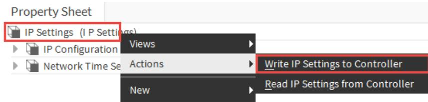
Fig. 132 Write IP settings to Controller
