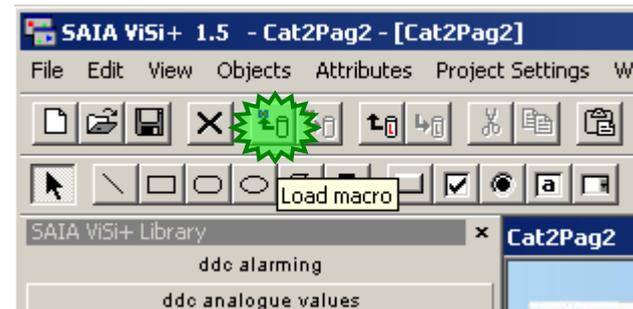
Select the macro we saved before: heat\_circuit.pmc and press “Open”
