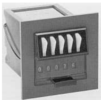
The fixing frame with clamping spring for plug-in mounting; connection by means of tags (2.8×0.8mm) for push-on connectors or soldering.
