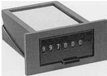
The fixing frame with clamping spring for plug-in mounting; connection by means of tags (2.8x0.8mm) for push-on connectors or for soldering.
