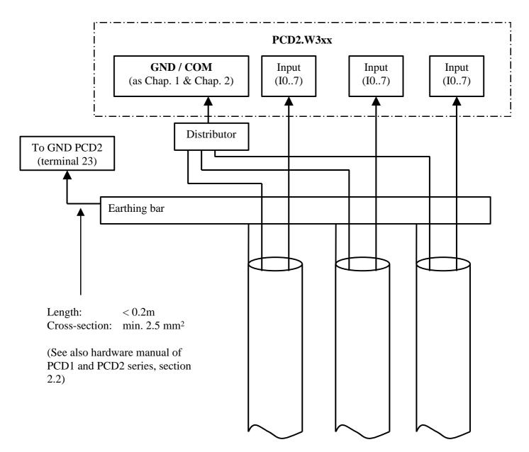
The earthing bar drawn above can also be used for other devices. The lower the impedance achieved when the screening is carried to the earth, the better that screening can fulfil its purpose.
