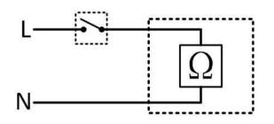
There are two cables, one is connected with live line, one is connected with neutral line, no color identification.
