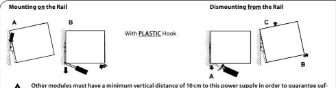
ficient auto convection. Depending on the ambient temperature and load of the device, the temperature of the housing can become very high!
