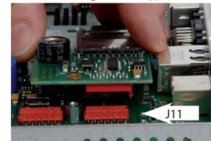
5. Screw the module to the screw supports.
