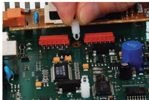
3. Align the red module connector with J11
