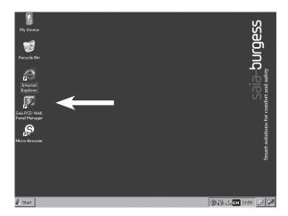
Activate the expanded view of the Saia<sup>®</sup> PCD Web-Panel Manager. A dialogue will appear asking for a password. In the default setting, no password is configured. Simply click OK.
