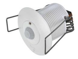
The SBC multi-sensor allows the comfort level of a building to be adapted according to the occupancy status of a room (motion detection), and the light intensity to be adapted through the luminosity sensor. The comfort parameters are controlled with the multi-purpose remote control or the CVC. It has an integrated Bluetooth transmitter/receiver.
