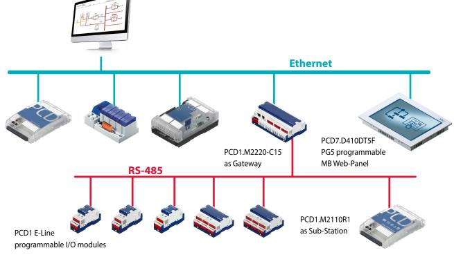
Ethernet communication to PCD's and on PCD's over RS-485 which are connected behind a gateway.
