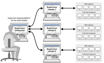
There are many different ways to split up a large installation. You should aim to configure each 'remote' Saia PCD® Supervisor station to have a near equal share of the processing overhead. For example, by allocating each PC to a separate floor or building, or dividing up the number of points or LANs. Remember to take account of any slower connections to remote sites or slower network media.
