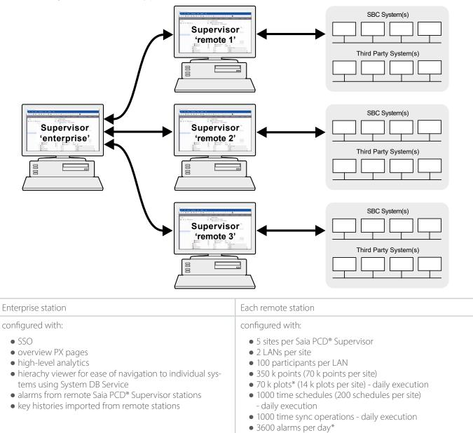
**Note:** Although tested using simulated only SBC systems, this configuration could accomodate other third party networks, e.g. PCD3.M6860, PCD3.M6893 and BACnet, without affecting the overall system performance.
