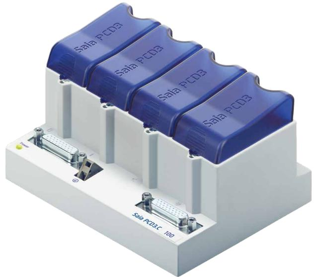
The PCD3.Mxxxx controllers can be expanded with PCD3.Cxxx components, making additional module sockets available. On the PCD3.Mxxx0, up to 15 PCD3.Cxxx module holders can be attached (PCD3.M3020/3120 cannot be expanded). This allows the user to attach a maximum of 64 I/O modules, or 1023 digital inputs/outputs.
