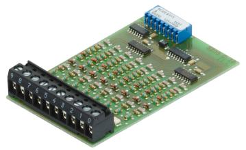
Low-cost input module for source or sink operation with 8 inputs, electrically connected. Suitable for most electronic and electromechanical switching elements at 24 VDC. The PCD2.E111 differs from the PCD2.E110 in its shorter input delay, typically 0.2 ms.
