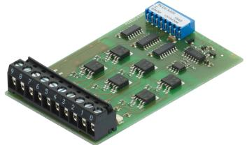
Low cost output module with 6 transistor outputs 5 mA ... 2 A, without short-circuit protection. The individual circuits are electrically connected; the voltage range is 10 ... 32 VDC.
