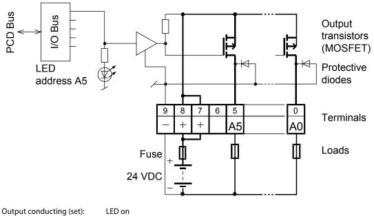
Output disconnected (reset): LED off
