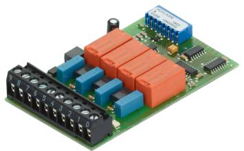
The module contains 4 relays with normally-open contacts for direct or alternating current up to 2 A, 250 VAC. The contacts are protected by a varistor and an RC element. The module is especially suited wherever perfectly isolated AC switching circuits with infrequent switching have to be controlled.
