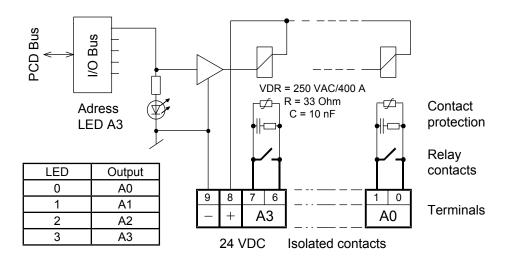
Relay energized (contact closed): LED on Relay reset (contact open): LED off 24 VDC must be connected to the +/- terminals.
