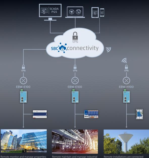
Remote monitor and manage properties Saia PCD controllers are securely connected to your VPN network via a LAN-LAN router.
