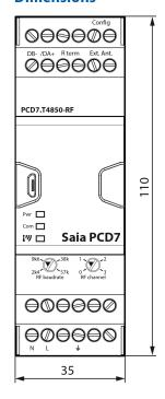
Housing width 2 TE (35 mm), electrical control cabinet compatible (in accordance with DIN43880)
