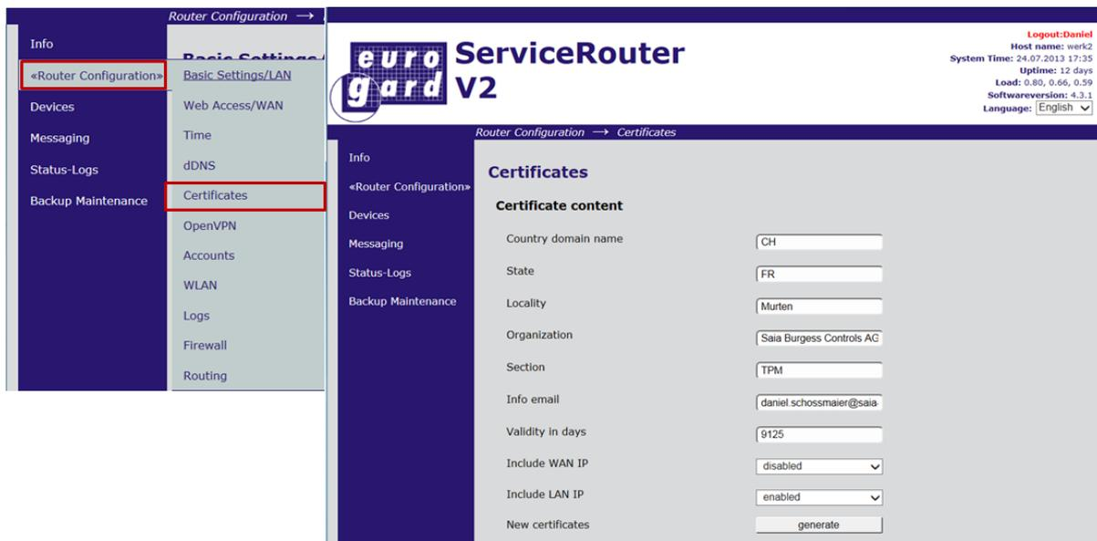
The screenshot shows the 'Certificates' configuration page in the ServiceRouter V2 web interface. The left sidebar is expanded to show 'Router Configuration' and 'Certificates'. The main content area displays the 'Certificate content' with the following fields:
