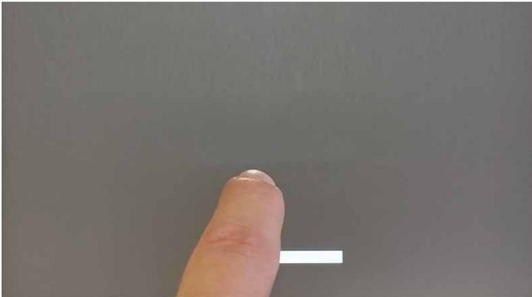
When “tap-tap detected” message appears on the top of the screen, wait for 5 seconds (without touching the screen) to enter System Settings sub menu
