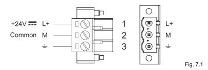
3 conductor 1,5 mm<sup>2</sup> wire size minimum, minimum temperature conductor rating 105°C.
