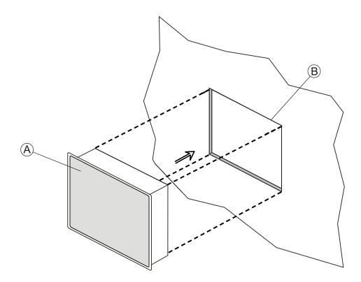
A. PCD7.D5xxCF B. Installation cut-out Safety instruction | Installation Procedure
