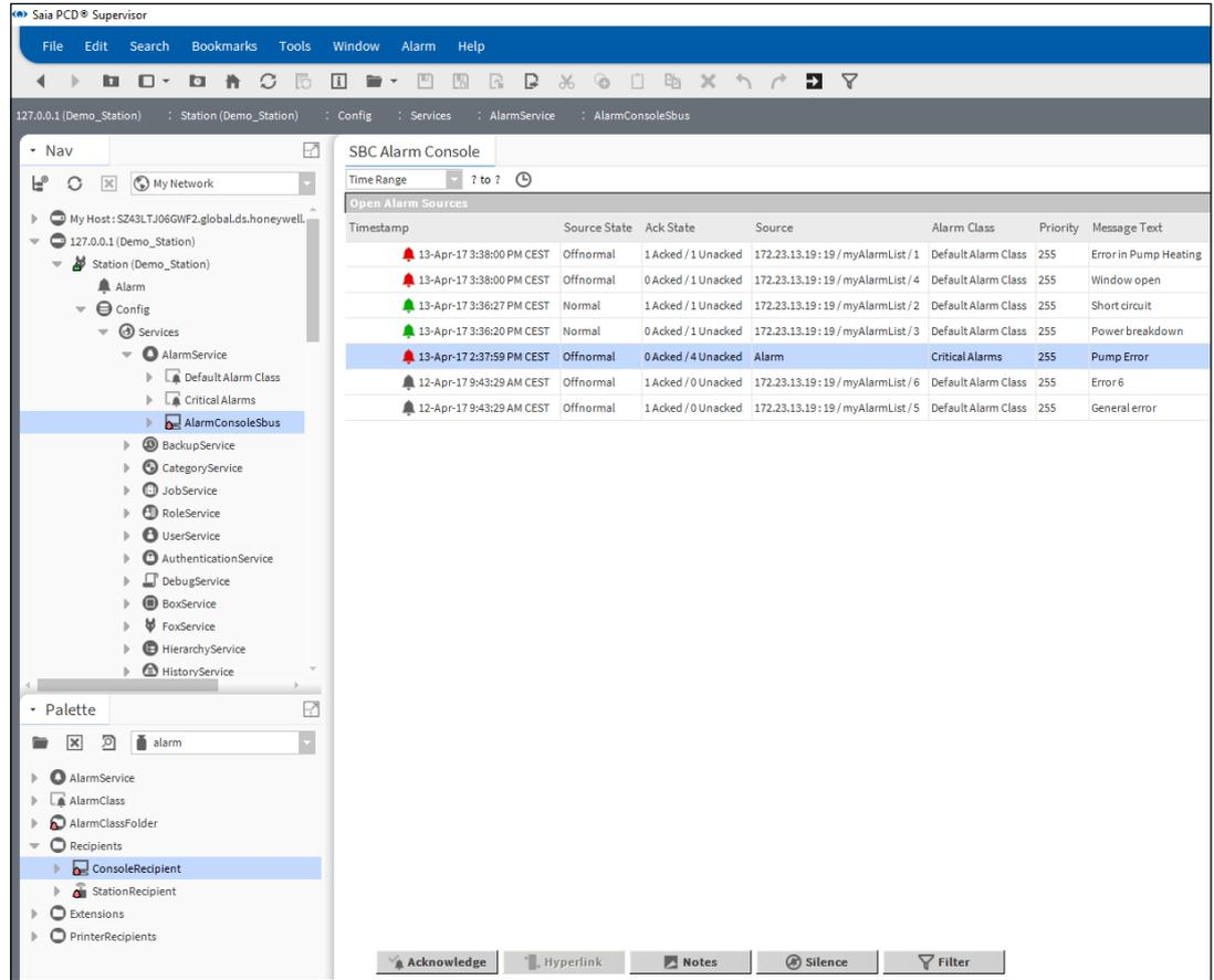
When new alarm comes there is an audible sound to indicate it. This feature can be deactivated with the Silence button.
