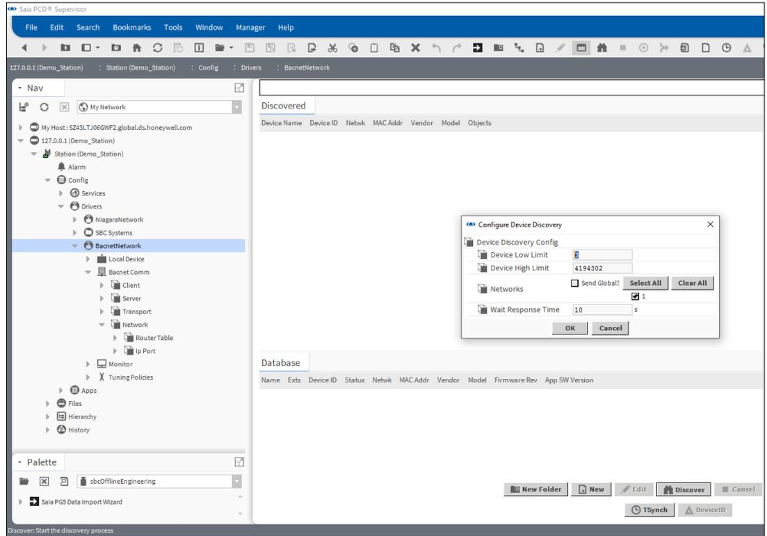
If the address range of controllers is known then the **Device Low Limit** and **Device High Limit** can be edited to reduce discovery time.
