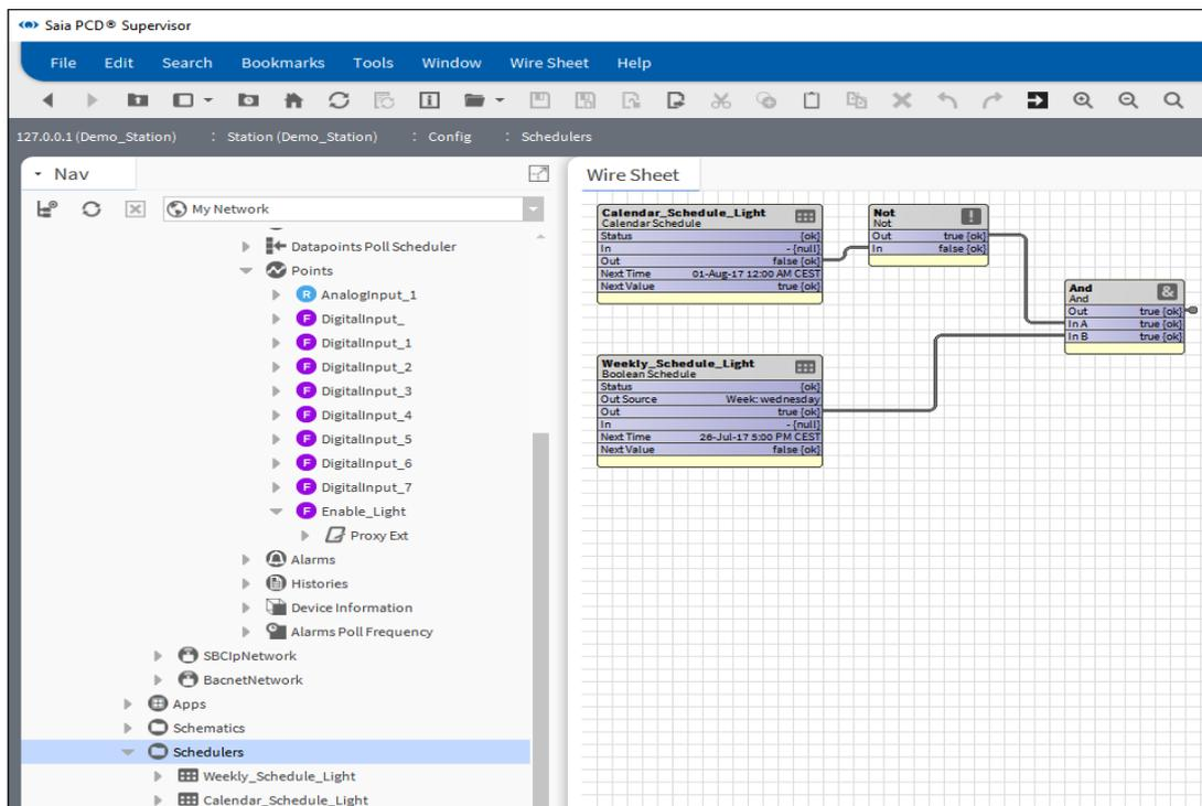
The **Out** pin of the And Function box must be connected to the Enable\_Light pin **IN16**. But these Function Boxes are located in two different Wire Sheets. We need to link these two pins together.
