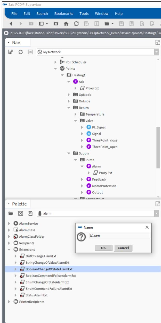
6. Set up the properties of the Alarm Extension
