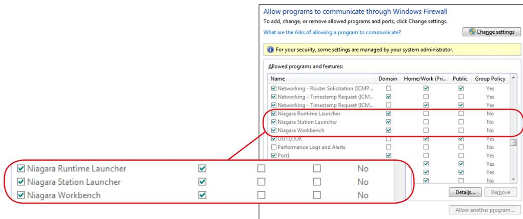
3. Scroll down the list and check that entries exist for Niagara Runtime Launcher, Niagara Station Launcher, and Niagara Workbench for your Saia PCD® Supervisor installation folder. If these programs do not appear in the list you will need to add them (see procedure below).
