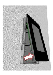
Lift the panel out of the adapter and ..
