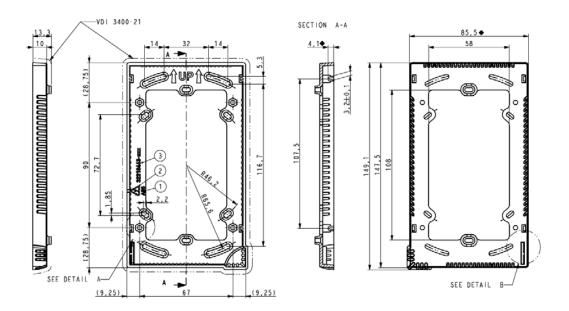
The adapter can be mounted on standard double wall installation boxes.
