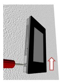
Press on the locking ratchet using a screwdriver and ..
