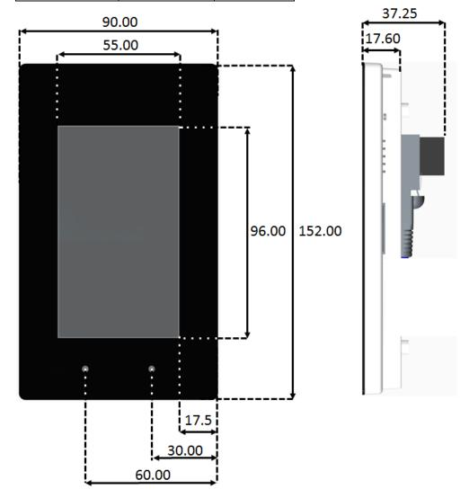
In the sideview can be seen, that some components are protruding out of the mounting frame. That means they go a few millimeters under the surface of the wall plaster.
