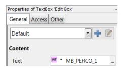
4) The user project must now use the MB\_PERCO\_1 variable when searching for the array. In order to do this, the symbolic name of the PCD variable must be searched for dynamically. In the web application, the internal variable must now be included in the resolution of the PCD variable.
