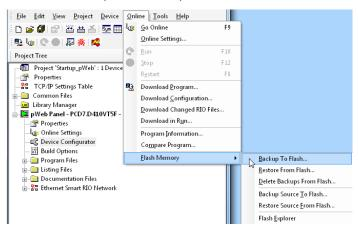
Because the user program is already backed up in the on-board flash memory, only RAM DB/texts of the on-board flash memory will be backed up (not visible to the user)
