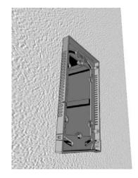
Screw the adapter onto the wall installation box ..
