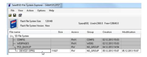
Exit the SD File Explorer and don't forget to **save the file**, in order to write the SD card.
