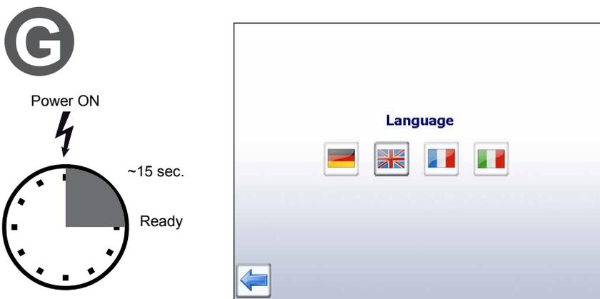
After connecting on power supply, an automatic search run (scan) of the connected S-Bus network is carried out immediately following a short initialization.
