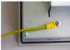
Protective earth must be connected!
