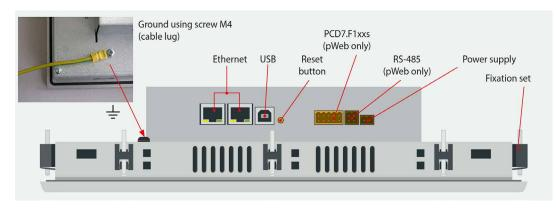
PROTECTIVE EARTH MUST BE CONNECTED!
