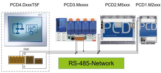
The pin nos of the connected PCD are explained in the respective manual.
