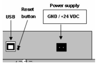
c) Switch on the MB panel with ON at the same time. Wait 3...4 sec. until the LED starts to flash.
