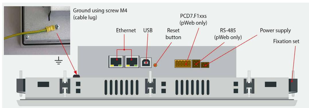
PROTECTIVE EARTH MUST BE CONNECTED!
