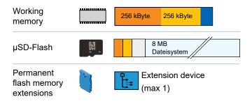
Memory structure of a PCD1.M2\_ with additional memory cards
