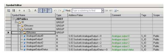
The analogue values shall be directly written in the AnalogueOutputx registers. Each channel will be updated after the last COB.
