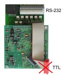
PCD2.T814: Analogue modem 33.6 kbps (RS-232 and TTL interface)
