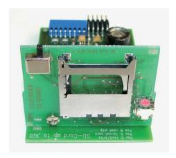
The PCD2.R6000 memory module is not supported on the PCD1.M2 $\_$  because the SD card cannot be mechanically secured.
