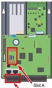
Terminal block X2 (connection terminals for Slot A)
