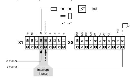
Input signals (always source operation): H = 15...30 VL = -30...+5 V or unconnected
