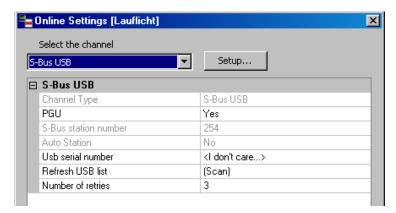
Activating the "PGU option" ensures that the PCD connected to the PC can be reached directly, independently of the configured S-Bus address.
