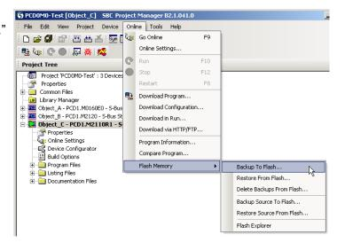
Since the user program is already stored in the on-board flash memory, only the RAM DB/text data from the on-board flash memory is backed up in the folder PLC\_SYS. This folder is not visible for the user. Access is not permitted.
