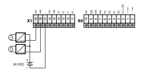
\* 4..20 mA through the user program or in the PG5 → Device Configurator → Media Mapping
