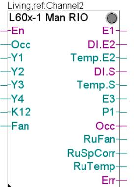
Instead of standalone control operation, internal regulation and control can also be completely disabled. The outputs are then dependent only on the communication master. For this RIO (remote input-output) operation, the RIO FBox is provided.
