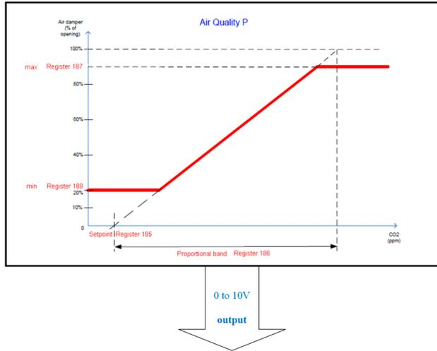
**In mode 2**, air quality demand and cooling demand can act on dedicated 0-10V output. The maximum between air damper demand of opening and cooling demand will be applied on the output.
