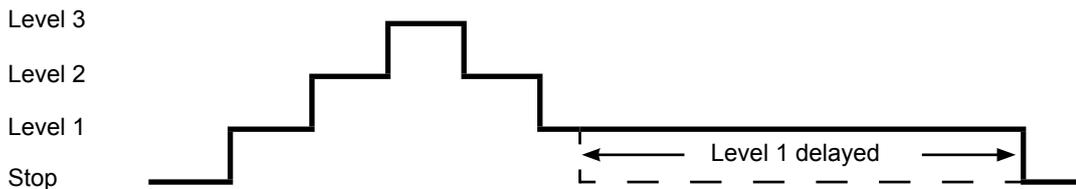
The system switches between steps automatically with no delay, until step 1 is deactivated. This deactivation is delayed by a configurable time. Settings are entered via the Config FBox or register 127, in 20-second steps.
