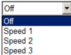
There are many reasons for limiting fan speed across the board. The minimum fan speed can be parameterised independently of the maximum level. If both values are equal, the fan always runs at the selected step level. For values Min = 0 and Max = 3, the controller selects the steps automatically without any restrictions. This parameter defines the behaviour after a restart without any manual intervention.
