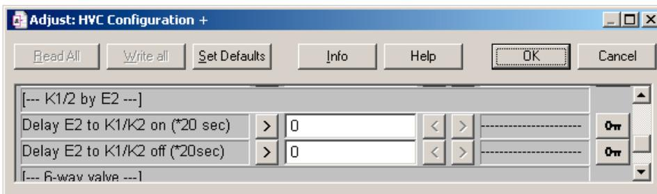
When the input E2 is configured as “K1/K2 via E2” (Register 10 = 5) this parameters will have an effect (See also 3.3.1.3 Hardware)
