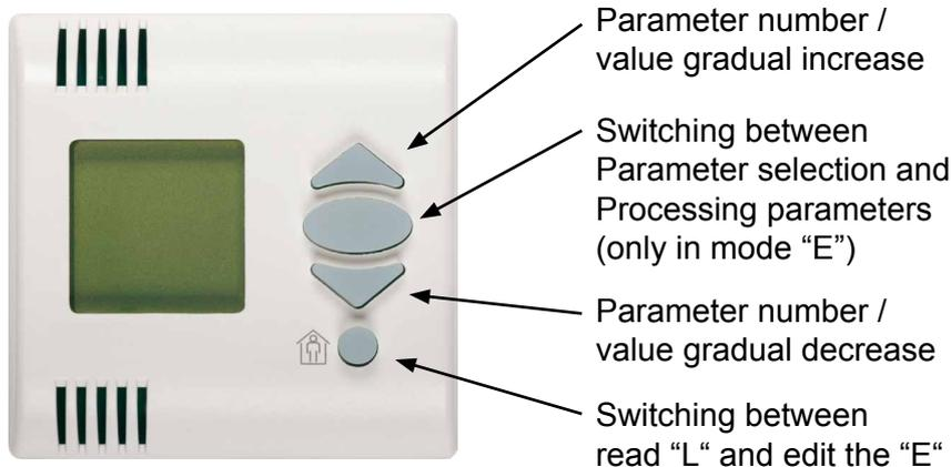
The small round button is used to switch between reading end editing parameters. The arrow keys are used to select the desired parameter. The parameter is retrieved with the oval key. Pressing the key again returns to the parameter selection menu.
