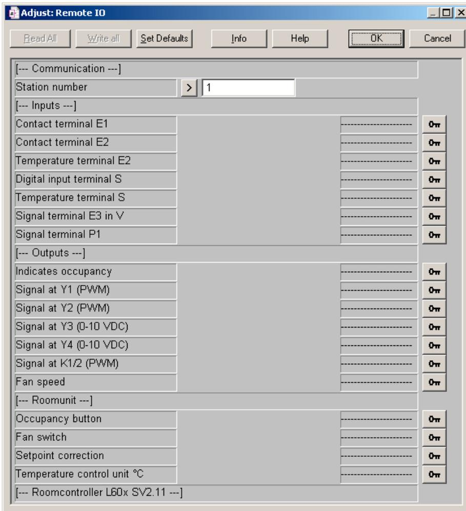
The RIO FBox switches the room controller into manual mode. This deactivates all independent control functions and the values at the FBox inputs are sent to the room controller.
