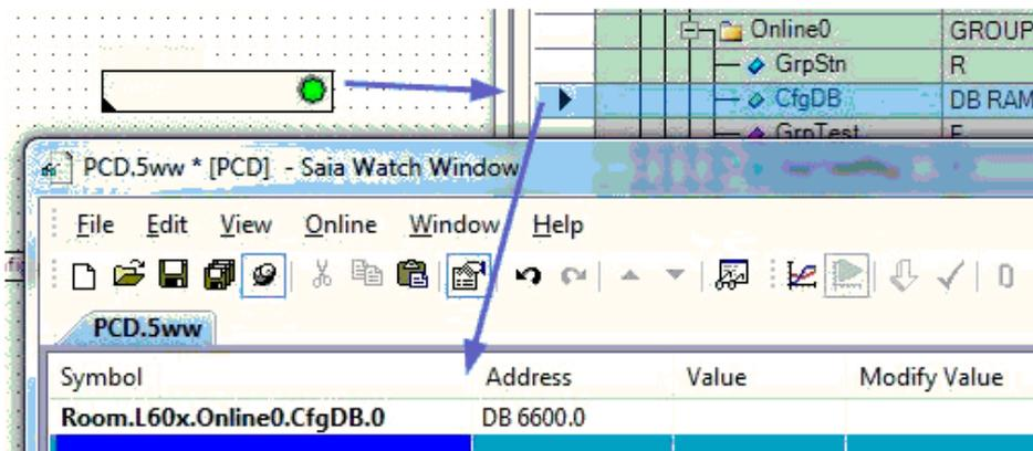
2. The entry in the WatchWindow ends with ".0" and represents the first element of the DB. The element no. 0 represents the station address 0. A separate entry must be displayed for each station address. Click into the field with the symbol name and add two periods (= marking for a range) and enter the last station address that is to be displayed directly behind without spaces; in the example, this is 32:
