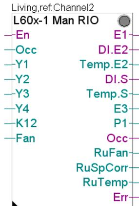
Instead of standalone control operation, internal regulation and control can also be completely disabled. The outputs are then dependent only on the communication master. For this RIO (remote input-output) operation, the RIO FBox is provided.
