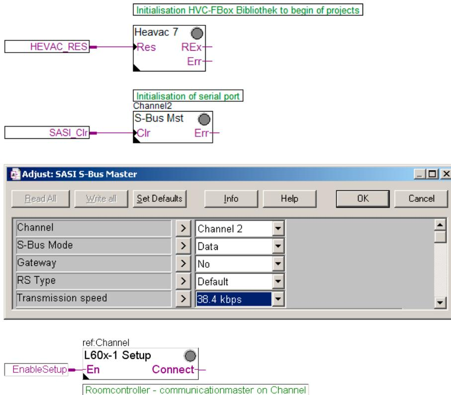
At start of project, the Hevac library and the serial interface need to be initialised. The picture shows the configuration for a PCD3 using the integrated serial RS-485 interface "Channel2".
