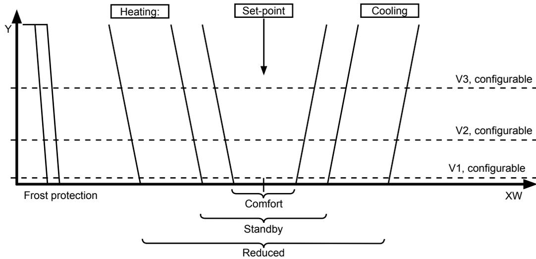
The room controller can work in one of the 4 operating modes “Frost protection”, “Reduced”, “Standby” or “Comfort”. The operating mode depends on the window contact, a preset value and the presence sensor.
