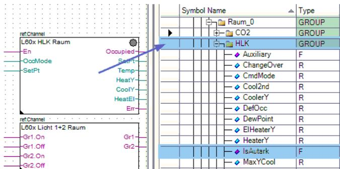
2. The symbol **IsAutark** can now be dragged into an output connector. If the switch can be made only through the door contact, this can be written directly (in the above example). If the switch must be made only once on changing the door contact, the contact plan-module must be processed with leading edges and set/reset (in the example below). In this way, it is possible if need be to change the current mode independent/as slave at a higher level.
