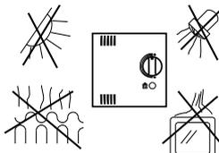
Do not install next to heat sources such as heaters, refrigerators, lamps etc.
