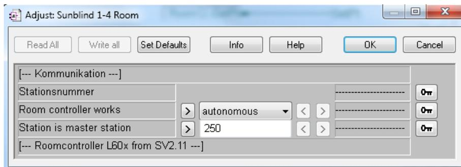
The FBox works on the "read/modify/write" principle. After a change of value at one of the FBox outputs, the current blind status is read from the controller. The information read is modified according to the changed inputs. Data where the associated FBox inputs have not changed are retained. The new status is then returned to the controller once more.
