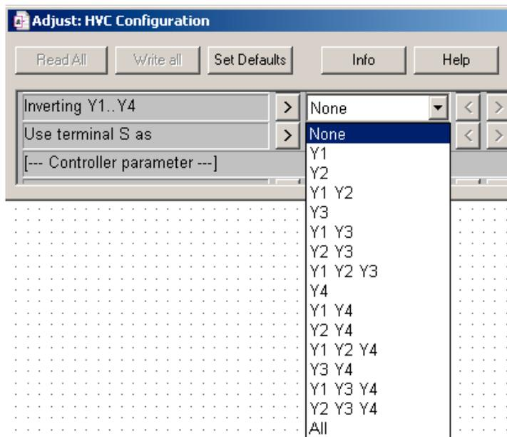
Up to FW Version SV2.12 this setting is not stored in the eeprom, after a power down it reset with the default value "None" (0).
