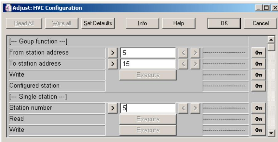
The configuration (read and write) of the room controller is performed online. It is also possible to configure a number of room controllers which have the same configuration on a single occasion, provided these are in a connecting address range (e.g. from address 123 to 167).
