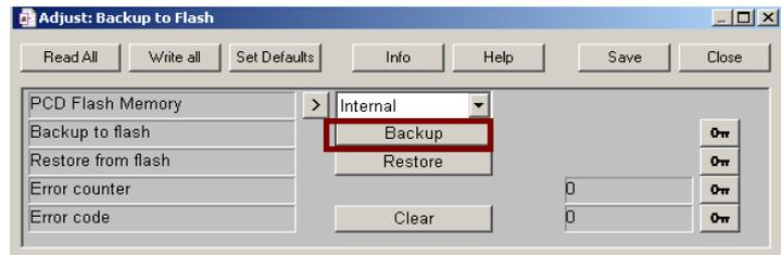
For a short time, "1" appears at the output of the "Backup to flash" FBox. This means that data has been backed up.
