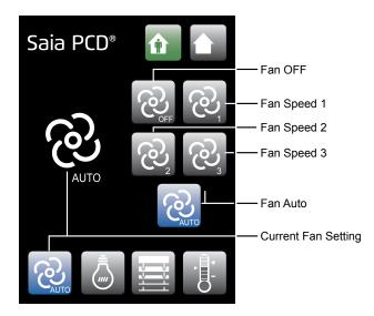
You can choose to set the fan at the speed you want (**Off**, **1**, **2**, or **3**) or to follow the automatic setting (**Auto**) which adjusts the fan speed depending on the gap between ambient and desired temperature.
