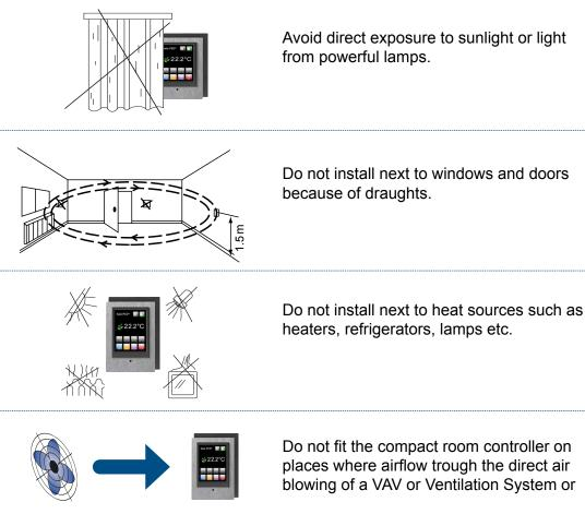
trough a downwind of cold air above the compact room controller exist.
