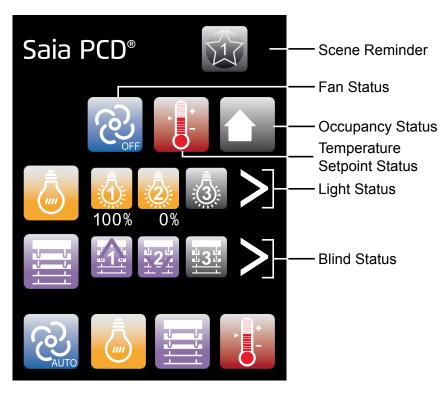
You can then adjust the different setting parameter. The parameters are automatically stored to the last value.
