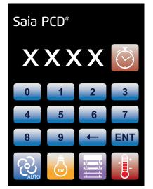
With the screen sleep timer you can set a time duration for screen turns off after a last action.
