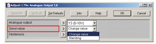
The internal parameter "Transmit value" is used to determine the communication behaviour of the FBox. The value at the input can be transferred to the room controller cyclically or only after a change of value.
