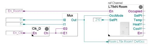
This can be useful if a timer clock or superior system is used for the changing of the operation mode.
