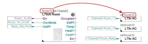
Free outputs, i.e. outputs not used by the selected application (see Configuration), can be controlled at will via the Saia PCD®. This requires the use of a Room FBox with a unique FBox name. The outputs are passed to the Room FBox by the analogue output FBoxes. The Room FBox is entered into the analogue output FBox as a reference. (See also "Function, manual output control".)
