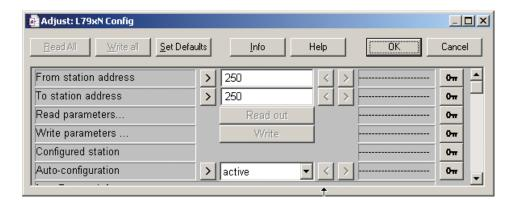
The compact room controllers can be parameterised very efficiently. Where a set of room controllers with consecutive S-Bus addresses are to be configured with the same basic parameters using the Autoconfiguration function, a single Config FBox can distribute the parameters to all the room controllers automatically. To do this, the start and end addresses are entered into the Config FBox in the "from station address" and "to station address" parameters and "Autoconfiguration" is set to "active".
