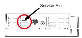
When the "Service pin" button is pressed, the compact room controller enables an additional station address 252 for a minimum of 15 minutes. The controller can use this address to communicate with the master independently of all other software components. Provided that the room controller is receiving telegrams via this address, the timer for time monitoring is restarted each time. Only when the timer expires (after 15 minutes) is station address 252 deactivated.
