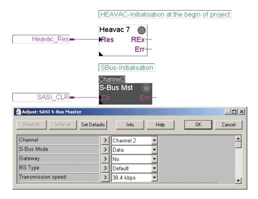
Initializing for the communications room controller must also set the FBox «L79x Setup» at the beginning of the program.
