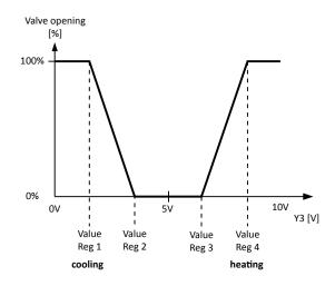
The voltage-level of the cooling and heating curve can be adjusted over 4 register values.
