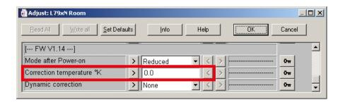
Note: This parameter is only applicable if the temperature sensor is selected as "L79x" (in the config-FBox)
