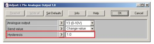
For a transfer after a change of value, the "Hysteresis" parameter defines the minimum change to the input value (compared to the last value sent) required to trigger a fresh communication.
