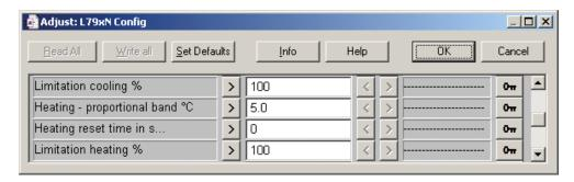
The current value is set in the Room FBox (register 142 for cooling and register 143 for heating)
