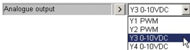
All outputs are basically analogue outputs. Outputs Y3 and Y4 work proportionally with 0-10 V. The switching elements such as Triac (Y1 and Y2) are operated by pulse width modulation (PWM). The cycle time is entered in the hardware settings. Values between 0.1 and 99.9 define the pulse/pause ratio. A value of 0 switches off a PWM output permanently, while 100.0% keeps it switched on.
