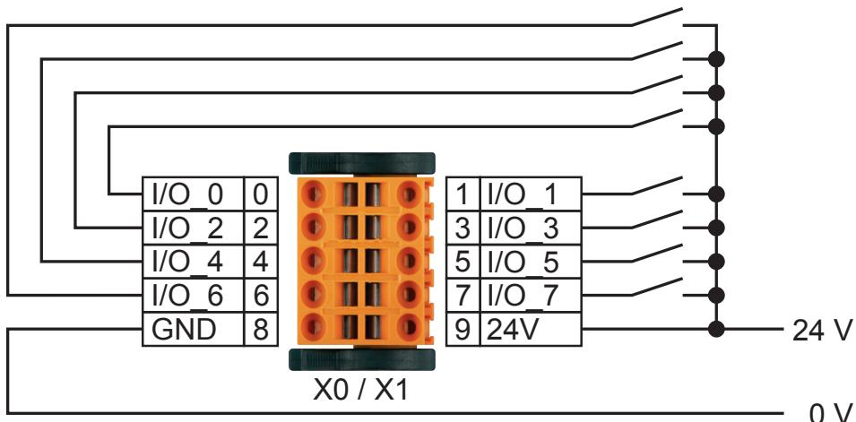
! The supply pins of each connector must be powered.
