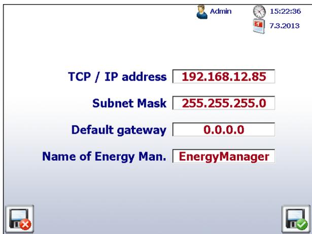
2. Assign the Energy Manager a unique address. The desired IP address can be set and changed at any time in the Energy Manager’s Setup menu. Navigation: Setup → TCP/IP
