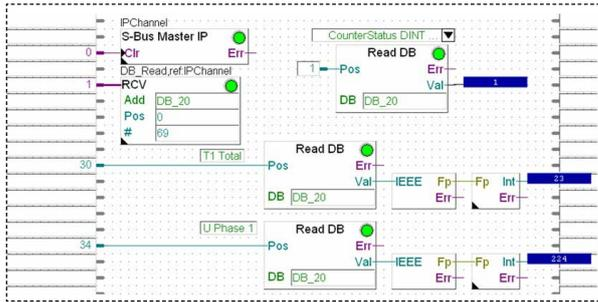
Each energy meter has its own database in the Energy Manager in which current values are saved. Chapter 15.1 provides an overview of the element addresses for the databases in the PCD “Database structure”.
