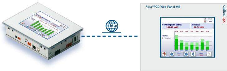
1. Using a network cable, connect the Energy Manager panel to the Saia PCD® Web Panel. See also Chapter 3.3 “Connecting the Energy Manager via the network”.
