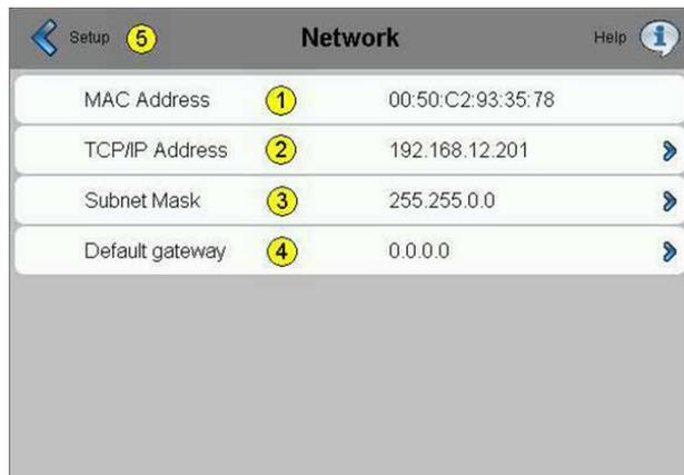
3. Configure the network by entering the Energy Manager’s IP address. Navigation: Panel Setup → Network → TCP/IP Address
