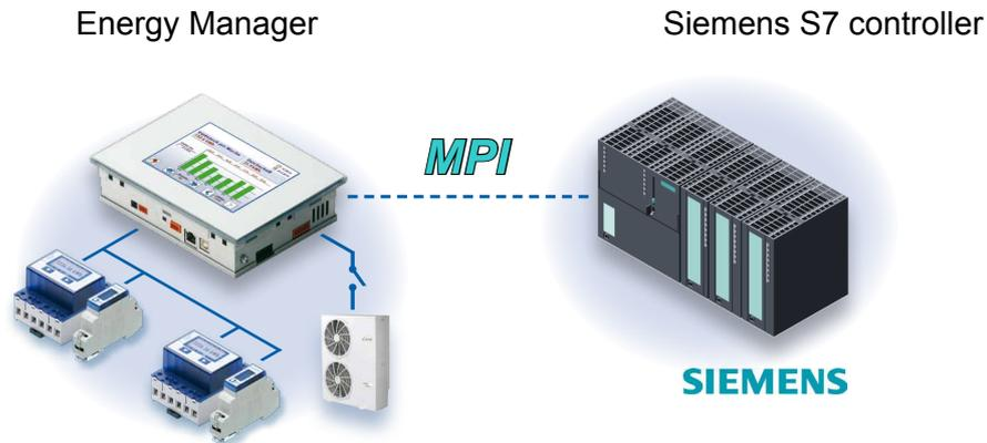
The Energy Manager panel has an MPI interface that can be used to connect a PLC in the RS-485 network. The Energy Manager has the MPI address 2.
