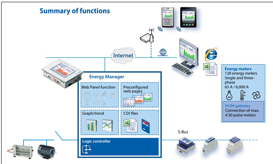
The user can execute logic applications in the Energy Manager and expand the control functions with remote data input and output. Flags, FCs, FB and DBs are available as resources. Since the SBC energy meter provides detailed information about every phase, the system makes it possible to not only optimise the use of energy but also to optimise maintenance and productivity.
