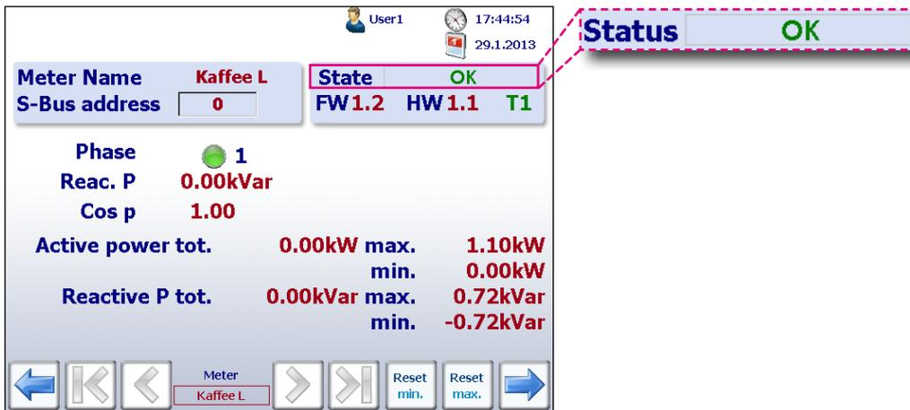
The Energy Manager designed for 64 subscribers makes it possible to group the energy meters. Up to 32 independent groups can be created. To add a meter, simply click on it in the configuration screen; this adds the selected energy meter to the group. To remove the meter from the group, simply click on it in the group. A group can also contain a group.
