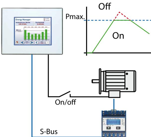
The average output over 15 minutes can be restricted automatically using the load dumping function.
