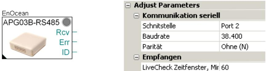
The FBox’s baud rate must match the baud rate set on the Omnio gateway device.
