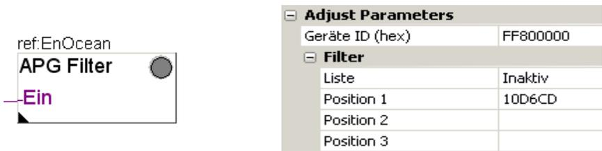
The gateway ID is entered in the “Device Identifier ID” field. Then the IDs of the sensors received by this gateway may be entered in the table. If the “En” FBox input is set, the FBox will transfer the list to the gateway.
