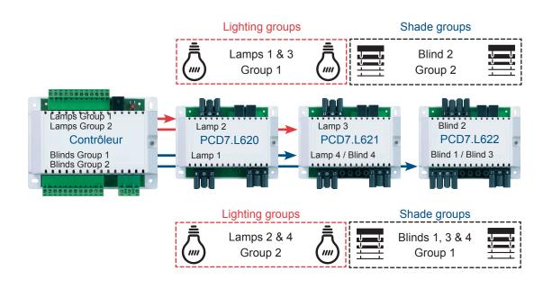
The PCD7.L611 integrates 4 light objects and 4 sunblind objects to manage these add-on modules.
