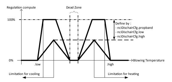
The blow limitation can only be used if a valid temperature is measured by the dedicated sensor, **nvoAuxSensor** different of 327.67°C (see chapter 4.1.2. Analogue inputs"). In this case, the limitation can be applied on heating, cooling or both application modes with the nciDischair.type.
