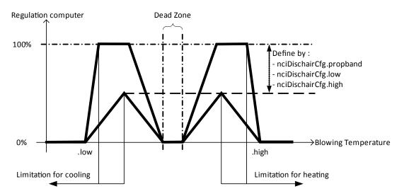
The blow limitation can only be used if a valid temperature is measured by the dedicated sensor, **nvoDischAirTemp** different of 327.67°C (see chapter 4.1.2. Analogue inputs"). In this case, the limitation can be applied on heating, cooling or both application modes with the **nciDischairCfg.type**.
