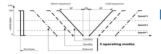
We can identify 4 different cases for the computation of the set point. The three first are "Comfort", "Standby" and "Reduced" mode and the last one is a specific application mode dedicated to the morning heating.
