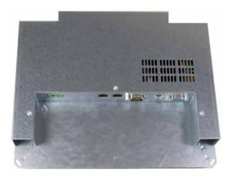
After removing the cover, the CFC slot is exposed on the top.
