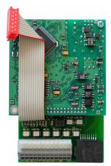
PCD2.T814: analogue modem 33.6 kbps (RS-232 and TTL interface) PCD2.T851: digital modem ISDN-TA
