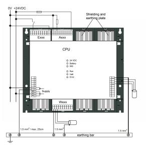
In the bottom part of the PCD2 module housing there is a shielding and earthing plate. Together with the shielding and earthing plate in the module holder, this constitutes the common, large-area ground for all I/O modules and for the external power supply.
