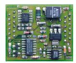
PCD7.F180: Connection module to MP-Bus The user can connect an MP-Bus line with 8 drives and sensors.
