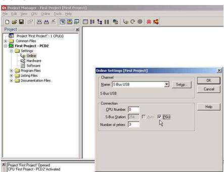
Onv connect the PCD to the PC via the USB cable. Ensure that the PCD is connected to the 24 VDC supply.
