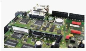
Push out pre-pressed aperture for the D-Sub socket and replace upper part of housing, section 3.5.4
