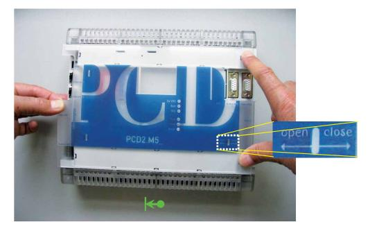
After removing the cover, the plug boards for flash cards, the lithium battery, the run/ halt switch etc. are freely accessible.
