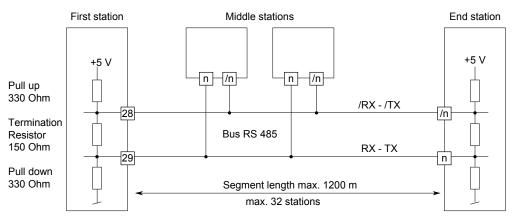
At the first and last stations, switch S1 must be set to "C" (closed). At all other stations, switch S1 must be left in position set to "O" (factory setting).
