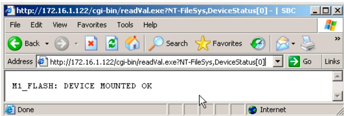
In case a writeable tag is to be written, the CGI command “writeVal” instead of the “readVal” will be used. The following example shows the sequence for checking the amount of freed blocks of the device mounted in slot M2 (→ address 1), launching a compression and then verifying the reduced amount of freed block:
