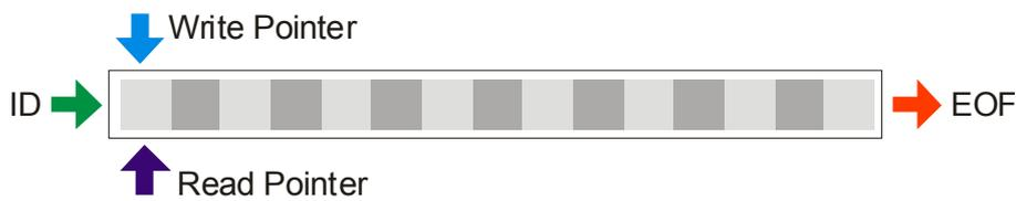
The pointers are modified by calling read, write or the seek function.
