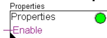
The FBox “File Properties” can be used to modify the configured values of the GroupID and the AccessGroup of the FBoxes accessing a flash device with file system.
