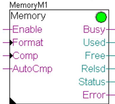
The “Memory Management” FBox must be placed before any other FBox that accesses the relevant flash device. In this FBox the GroupID for all created files on the flash device as well as the AccessGroup for the operations (create, delete, rename, read, write etc.) are configured.
