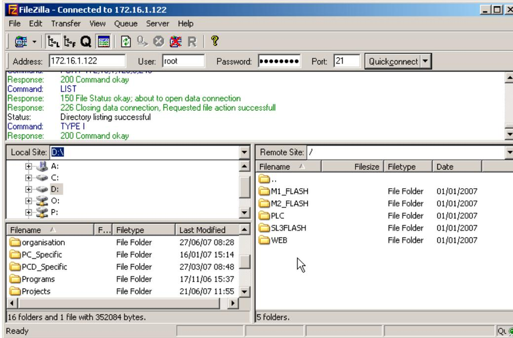
**Mx\_FLASH:** M1\_FLASH or M<sup>n</sup>\_FLASH. This are the drives representing the flash card(s) PCD7.R5xx plugged in the M1 or M2 slot of the PCD3. M5xxx or of the PCD2.M5xxx. The slot number is indicated at the beginning of the drive name.
