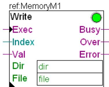
Write a record from a Saia PCD® media (Flag, Input, Register etc.) to a file. There are three FBoxes with that functionality (“Write Binary”, “Write Integer” and “Write Float”).
