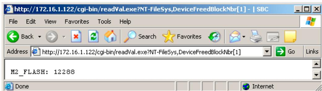
The example above is just a demonstration of the file system management on a Saia PCD® using CGI calls. Of course it is far more comfortable using these calls directly from an application (e.g. Visual Basic) or from a web page.
