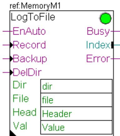
This FBox writes data in plain text into the specified file on the file system. The recording can be automatic at predefined interval.
