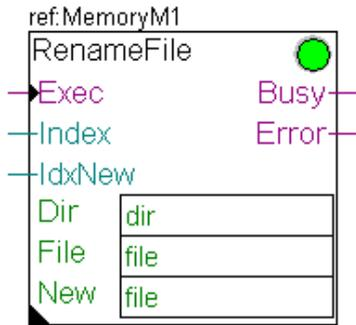
This FBox renames a file on the on the file system. The full path of the directory, the file to rename and the new file names must be entered in 3 Saia PCD® texts. The original and the new file names can be extended by an index. The original file gets the common file properties of the referenced FBox. The properties of the new file name (index and extension) can be adjusted in the FBox.
