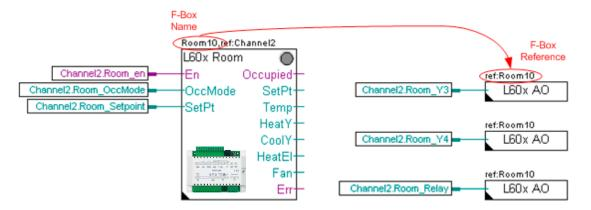
Free outputs, i.e. outputs not used by the selected application (see Configuration), can be controlled at will via the Saia PCD®. This requires the use of a Room FBox with a unique FBox name. The outputs are passed to the Room FBox by the analogue output FBoxes. The Room FBox is entered into the analogue output FBox as a reference. (See also "Function, manual output control".)
