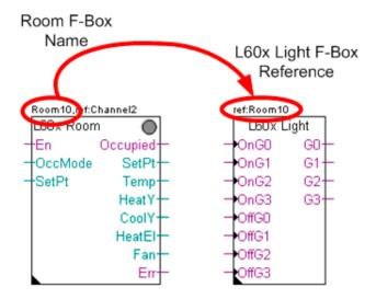
The "L60x Light" FBox can be used to switch up to 4 independent light groups. The individual light outputs are assigned to the groups in the configuration. See section on "Function, settings, light"
