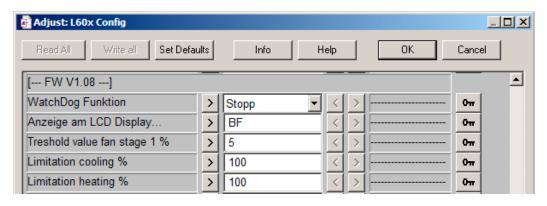
The current value is set in the Room FBox (register 142 for cooling and register 143 for heating)
