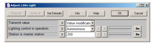
The FBox inputs only react to a change of value. The internal parameter "Send value" currently has no effect. To assure compatibility with future versions, "Value change" should be set.
