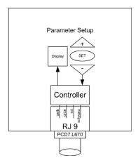
Local parameterisation aid in the form of a room control unit with RC-Bus interface to read and modify parameters. The PCD7.L679 communicates directly with the room controller and can be used for parameterisation anywhere there is no available network connection to a higher-level control system.
