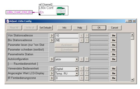
The room controllers can be parameterised very efficiently. Where a set of room controllers with consecutive SBC S-Bus addresses are to be configured with the same basic parameters using the Autoconfiguration function, a single Config FBox can distribute the parameters to all the room controllers automatically. To do this, the start and end addresses are entered into the Config FBox in the "from station address" and "to station address" parameters and "Autoconfiguration" is set to "active".
