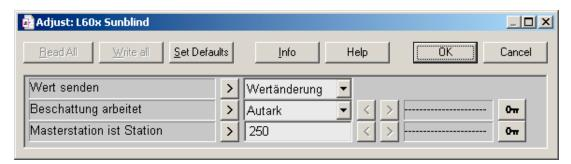
The FBox works on the "read/modify/write" principle. After a change of value at one of the FBox outputs, the current blind status is read from the controller. The information read is modified according to the changed inputs. Data where the associated FBox inputs have not changed are retained. The new status is then returned to the controller once more.
