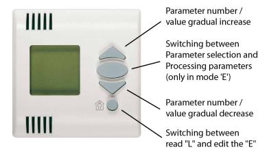
The small round button is used to switch between reading end editing parameters. The arrow keys are used to select the desired parameter. The parameter is retrieved with the oval key. Pressing the key again returns to the parameter selection menu.
