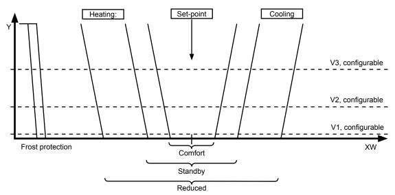
The room controller can work in one of the 4 operating modes "Frost protection", "Reduced", "Standby" or "Comfort". The operating mode depends on the window contact, a preset value and the presence sensor.
