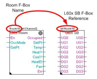
The "L60x SB" FBox can be used to switch up to 4 independent blind groups. The individual up/down outputs are assigned to the groups in the configuration. See section on "Function, settings, blinds"
