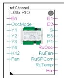
Instead of standalone control operation, internal regulation and control can also be completely disabled. The outputs are then dependent only on the communication master. For this RIO (remote input-output) operation, the RIO FBox is provided.
