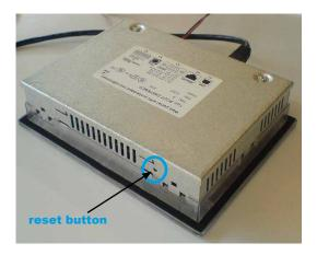
C. Then at the same time Power ON the MB-Panel. Wait about 3-4 sec. until the LED is flashing. Then go back to upper chapter 5.
